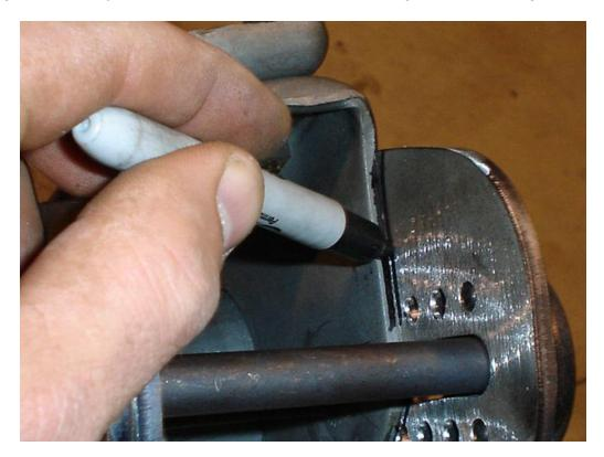
Next, use a ¼-inch drill and use the guide holes in the brackets to drill locating holes in the stock lower control arm perch. Once you have drilled all 4 holes, remove the instant center brackets.
