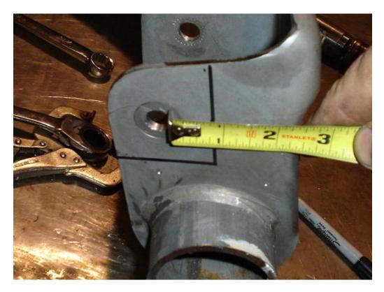
Using a 6'' cut off wheel, remove the marked sections of the old lower perch.
