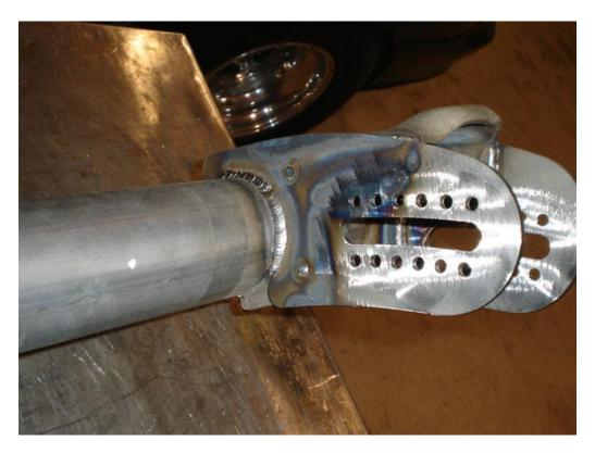
Make sure to weld the brackets on the inside and outside but be careful not to fill any of the retaining washer pin holes when welding the inside.
