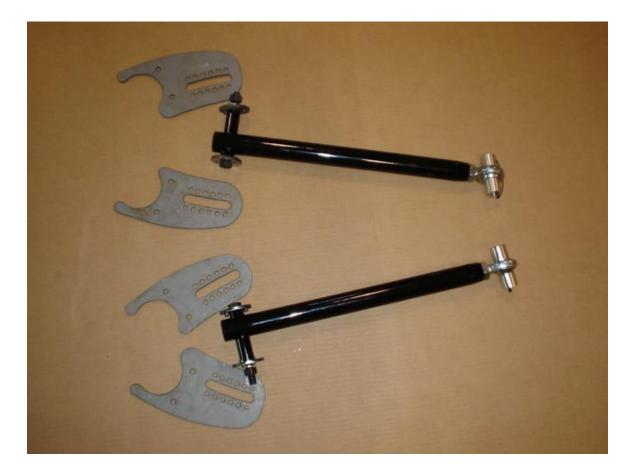
The first step would be to thoroughly clean your housing around the lower control arm brackets make sure to strip any paint and remove all grease and oil so the new brackets can be welded.
