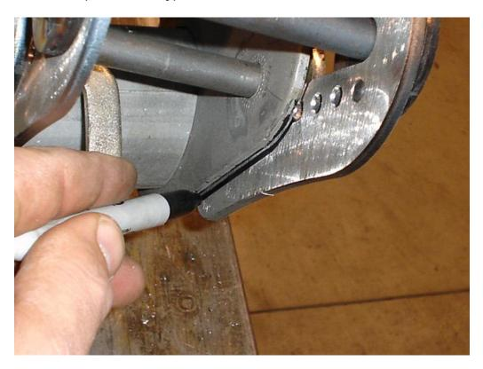
Make sure to go all the way around so the brackets can be realigned for welding.
