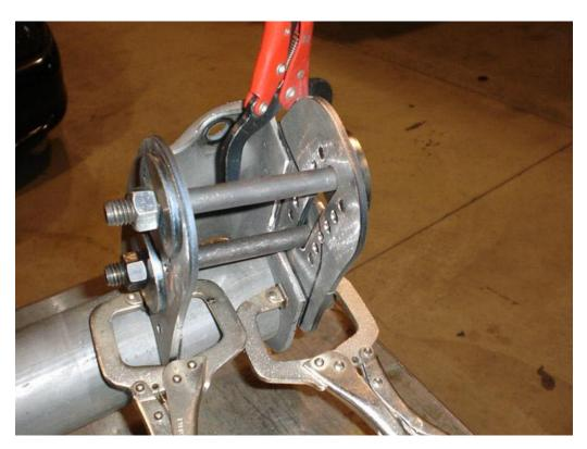
Make sure everything is lined up and that the bolts will move in the same plane, then tack weld the brackets into place and double check that nothing has moved. Weld the inside and outside of the brackets.
