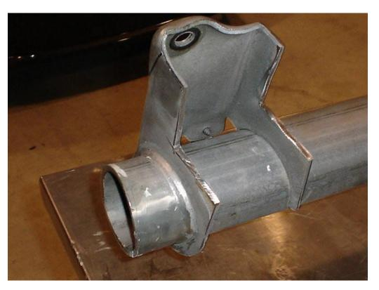
Using your guide lines and pilot holes, reinstall the inner and outer brackets, bolts and retaining washers.
