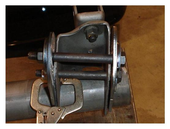
Next, take one inner and outer bracket (outer brackets are bigger) and bolt them in place using the supplied hardware and retaining washers. Use one bolt and 2 retaining washers in the stock hole and the other bolt and 2 retaining washers in the last hole on the brackets as pictured above. Use vice grips or c clamps to help hold the brackets in place.
