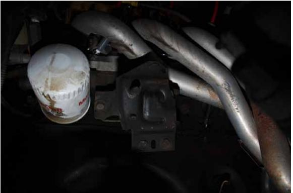
5. Remove the 2 bolts holding the mount to the engine.
