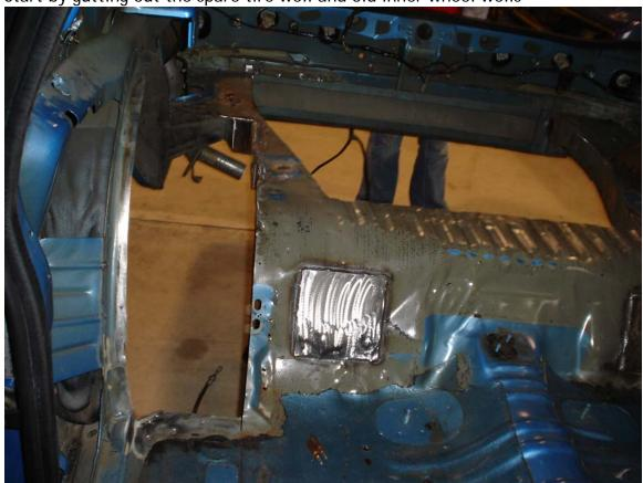
Cut along the frame rails for the spare tire well and measure 9" out from the pinch weld on the stock tub on the front and rear to mark your cut line.
