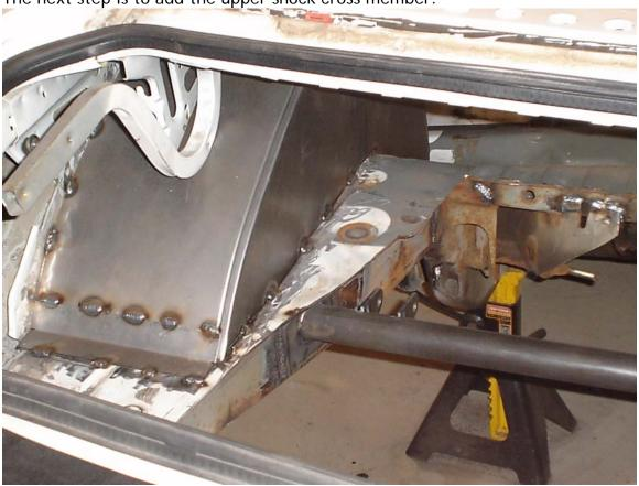
The upper shock cross member is already pre-assembled. Just hold it in place and measure from side to side to make sure it's square then tack it in place and double check your measurements. If it is in square, finish welding it in.
