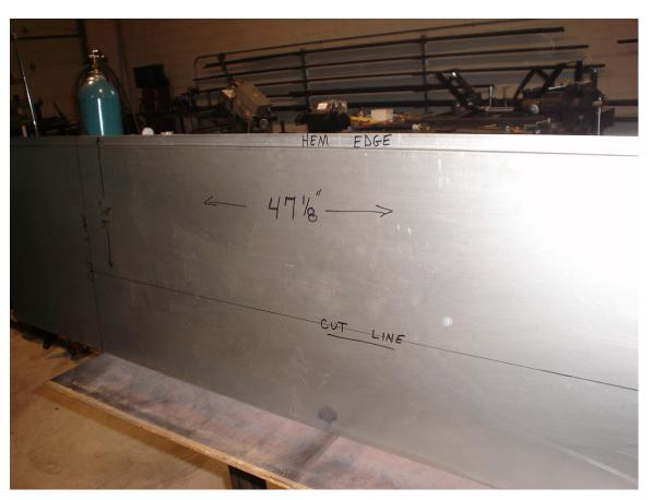
Once you cut out the flat part and inner part to fit your car, assemble the Pittsburg seam.
