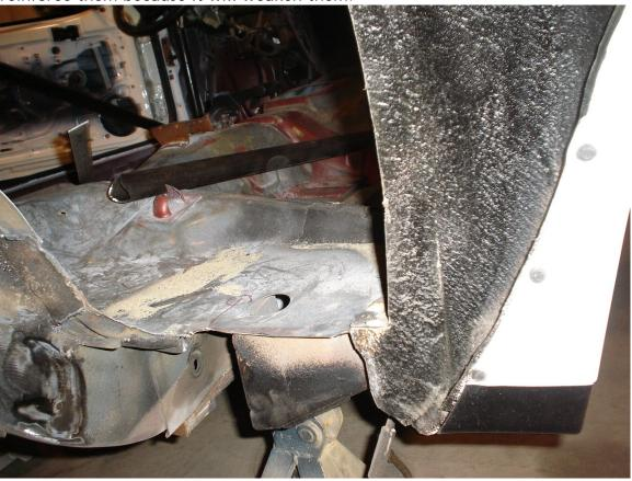
The next step will be to plate in the rear frame rail where it has been notched. We use 1/8 inch steel and MIG the plates in like this.
