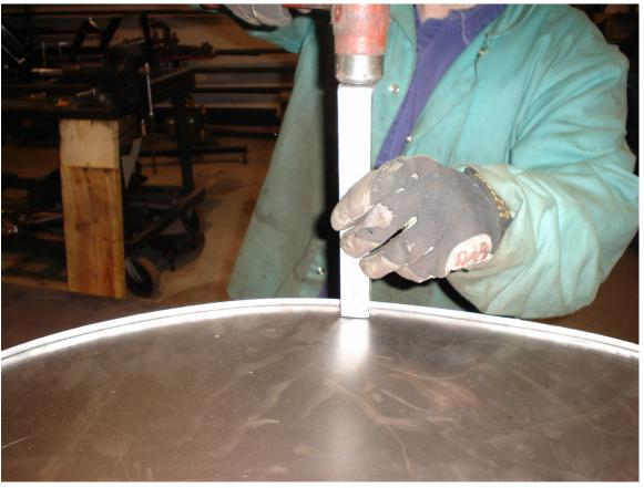
Use a piece of square stock to fit the lip into the receiver groove to make sure the seam completely locks.
