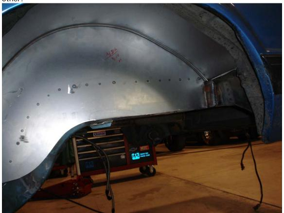
Fit the tub in and spot weld all the way around the tub.
