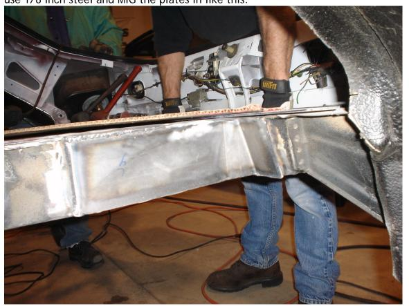
The next step is to measure out your mini tub to cut and fit it to the car. We leave a lot of extra material due to inconsistencies in tub sizes from year to year. It's always a good idea to make a cardboard template so your tub will fit right the first time.
